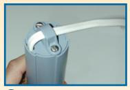
Secure wire clamp on bottom of tube.
