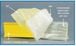
A surface veil is applied during the pultrusion process to ensure a resin-rich surface for superior corrosion resistance as well as an ultraviolet exposure barrier.
