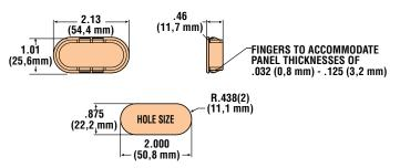
Material Polycarbonate Flammability Rating 94V-2
