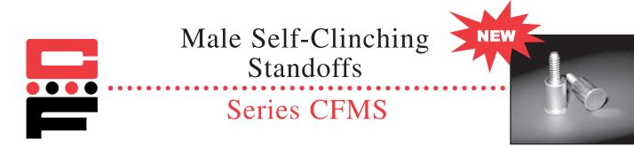
CFMS Standoffs provide a permanently captivated fastener with a reusable threaded post to mount PC boards and other components in electronic displays. The unique part is available in heat-treated and zinc plated steel or passivated stainless steel and can be installed into metal sheets as thin as .050 in (1.27 mm) thick.
