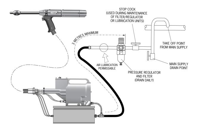
Follow the steps below when connecting the tool to the intensifier and main air supply:
