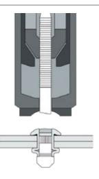
A spline feature on the pin comes into contact with a step on the sleeve creating an interference lock between the pin and sleeve and the pin breaks. The pin will break close to flush in minimum grip and below flush as the grip increases.
