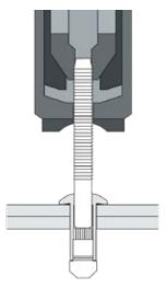
Insert the fastener into the hole and slip the installation tool over the pintail.
