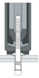
Press the trigger to initiate pulling action. As the tool pulls on the pintail, the solid pin head captures the end of the sleeve and acts to initiate bulb formation and draws the work pieces together.
