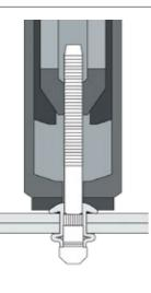
Continued pulling on the pintail expands the bulb to maximum allowable diameter.
