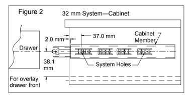
3. Use only the 32 mm system holes or the wood screw holes located at the tip of the breathing tabs. Do not use any other holes on the cabinet member for mounting (Figure 3).
