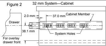
Use only the 32 mm system holes or the wood screw holes located at the tip of the breathing tabs. Do not use any other holes on the cabinet member for mounting (Figure 3).
