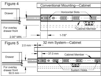
8. Use only the 32 mm system holes or wood screw holes located at the tip of the breathing tabs. Do not use any other holes on the cabinet member for mounting (Figure 6).
