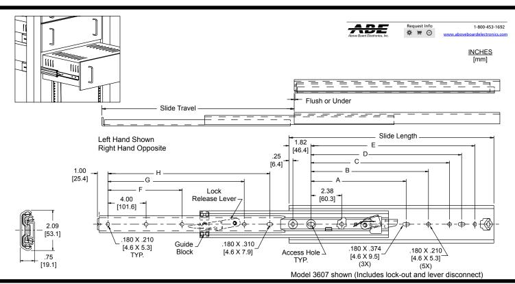
FinishClear zinc (C)TravelFull ExtensionLengthEven lengths12" to 28" [305 mm-711 mm]MountingBracket or side/hard mountHeight2.09" [53.1 mm]Hardware#8 pan head screws
